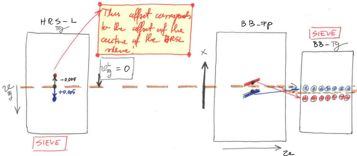
We can see, that if we make a narrow cut around  $|Tg z_L| < 0.002$ , we see two shapes in  $F_p - x, z_p$  plot, which correspond to two lines of holes. This suggests that the central line of holes of the BB sieve is not in the middle, but is shifted for approximately  $1/2$  of the spacing between the holes!
