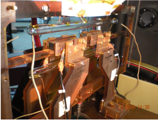
Figure 5: Left: Polarized ^3\text{He} cell mounted on the target ladder inside the target enclosure. Right: Schematics of the target cell. It consist of two main parts: the oval main target cell, which is put into the beam line and where the reactions happen, and a spherical pumping chamber (positioned outside the beam line) where incident laser light hits the ^3\text{He} gas and polarizes it.
