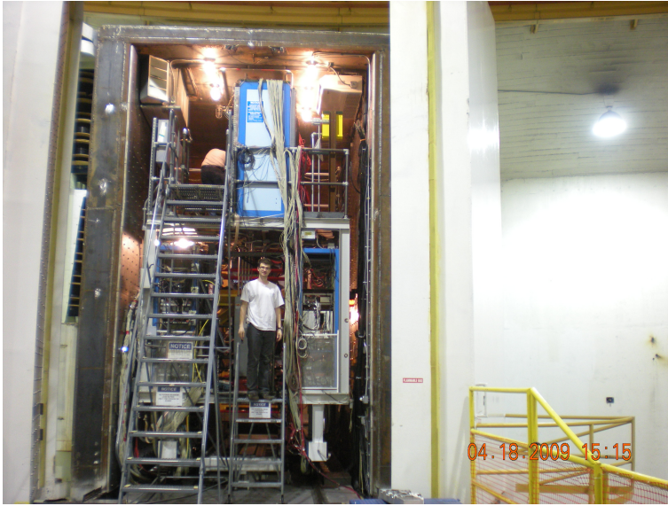
Figure 4: The figure shows open detector hut of the HRS-L spectrometer with the detector packages and electronics in it.
