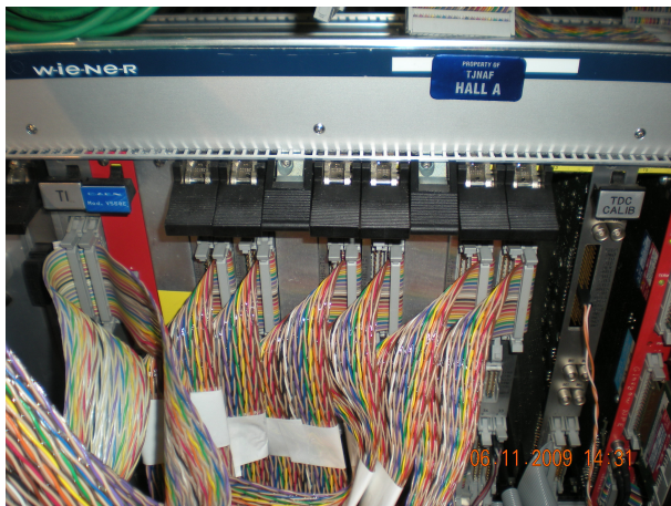
Figure 12: Left figure shows BigBite high resolution TDC modules. Right figure shows CEAN ADC modules
