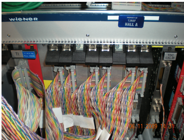
Figure 12: Left figure shows BigBites high resolution TDC modules. Right figure shows CEAN ADC modules
