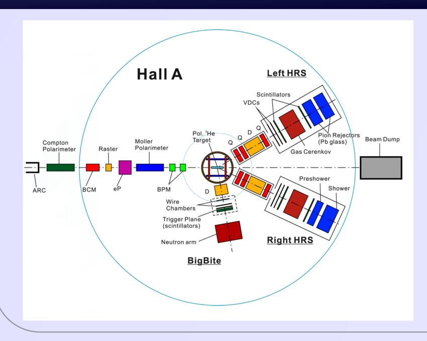
The instrumentation in Hall A [6] was designed to study electro- and photo-induced reactions at very high luminosity and good momentum and angular resolution. The central components of Hall A are two high-resolution spectrometers with the momentum resolution better than  $2\times 10^{-4}$ . The research program is aimed at a variety of subjects, including nucleon form factors, nucleon electromagnetic and spin structure fuctions, and properties of the nuclear medium.
