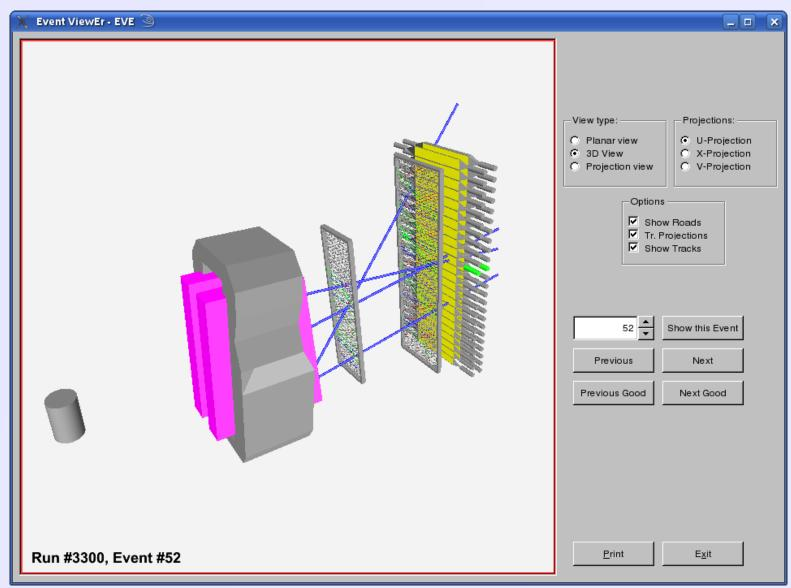
EVe is highly configurable event display for the BigBite spectrometer. It displays hits in scitillation planes and wire-chambers and shows all possible particle trajectories through the detector package.
